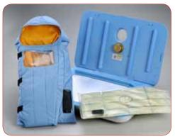
pouch is heated for 30 mins in the heater (second version uses boiling water instead of electrcity to heat) and then placed in the sleeping bag. It maintains the WHO recommended temperature of 37 deg C for 4-6 hours, after which it can be reheated.
