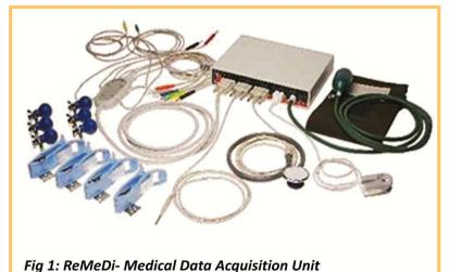
of various vital parameters about the patient to a doctor that are needed to make a decision on the preliminary diagnosis. The device was designed to measure six vital parameters such as Electro cardio graph (ECG), Blood pressure, Body Temperature, Heart Sounds, Oxygen Saturation (SPO<sub>2</sub>), Heart and Pulse rate. As a first step, the group
